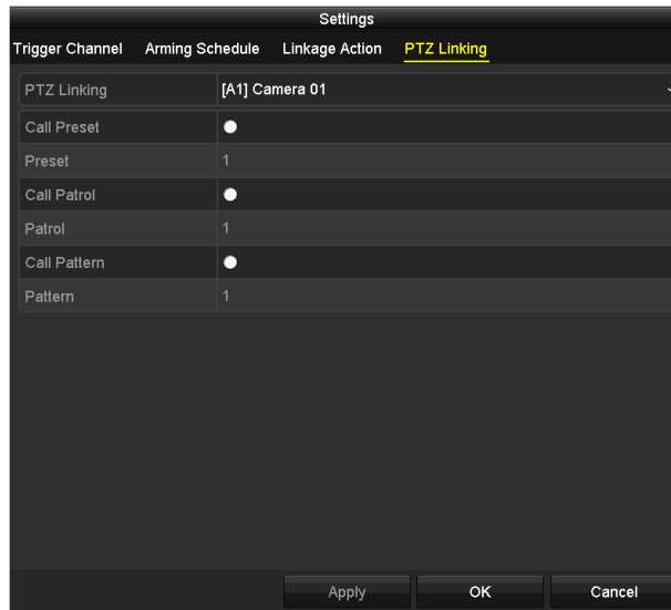
Figure 8-7 Set PTZ Linking of Alarm Input
